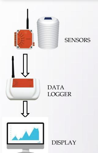
Allsolus is a Data Collection, Storage and Display system for the purpose of monitoring energy, gas, water.
