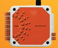
The AllSolus MeterLink is a compact power-monitoring device measuring power consumption for electrical, gas and water metering outlets.
